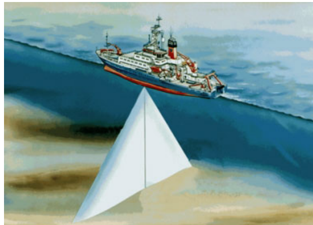
Hydrographic survey with multibeam echo sounder
